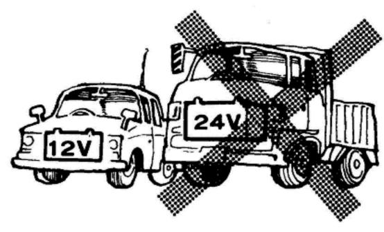
For mobile operation, connect the unit to a 12V car battery (6A). Do not connect it to a 24V battery.
