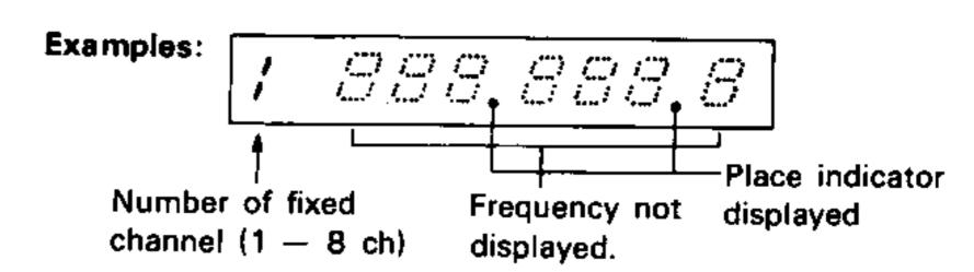
The channel number advances by 1 channel whenever the FIX CH switch is pressed. By holdingt the switch down, it advances continuously at about 0.5 seconds intervals, while a tone pulse is heard at each channel.
