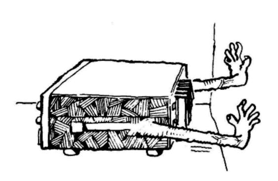
The TS-770E has a heat sink on the rear panel. Be sure to install the unit so there is adequate clearance at the rear and bottom.
