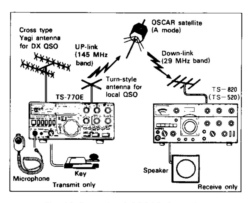
Fig. 16 Example of OSCAR Operation
